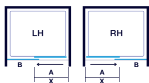
Sliding Door in Recess
