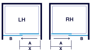
Sliding Door in Recess
