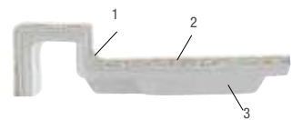
1. Top Acrylic capped ABS layer 2. Stone Resin 3. Bottom ABS layer (encapsulates the tray)
