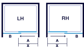
Sliding Door in Recess
